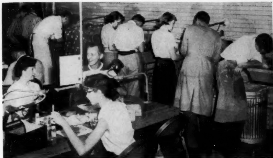
A portion of the battery of grinding wheels in the Green Briar Lapidary Shop in the Green Briar Field House, where wheels ranging in coarseness from 80-grit to 400 are used to bring agate, jade, carnelian, and many other types of semi-precious gemstones from roughly sawed shapes to finished ones, ready for sanding, polishing and mounting into jewelry. In the foreground hobbyists are enameling copper ornaments.
